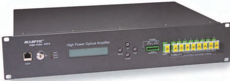
Figure 5.21. Example of a multiport optical amplifier (Alloptic).
